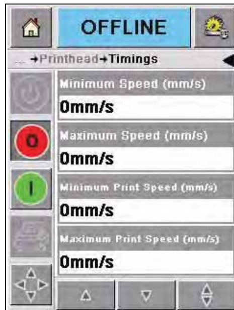
Figure 4-19: Printhead Timings Diagnostics Page
