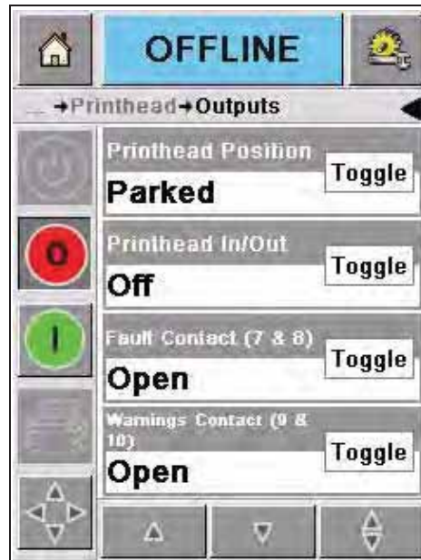
Figure 4-12: Printhead Outputs Diagnostics Page
