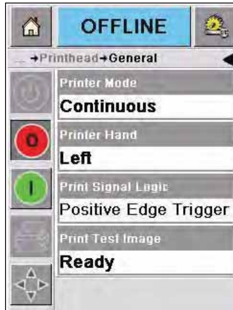
Figure 4-14: Printhead General Diagnostics Page
