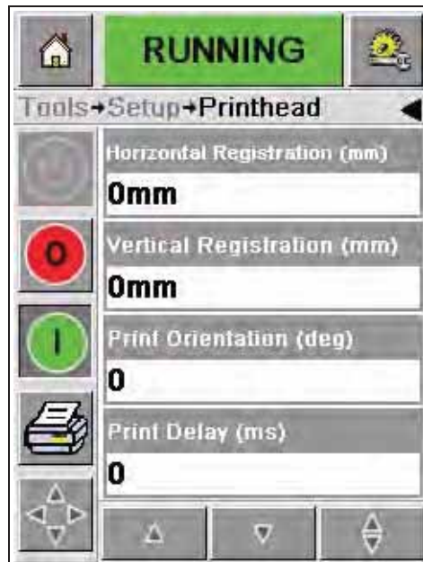
Figure 4-4: Printhead Parameters in Intermittent Mode
