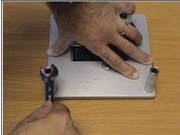
Figure 5-25: Roller Guide Removal
