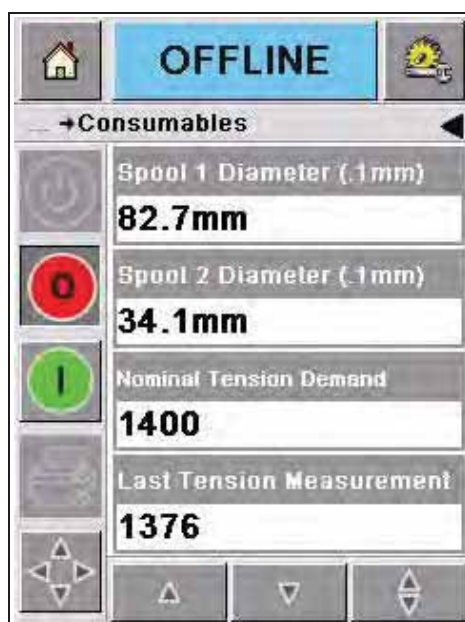
Figure 4-20: Printhead Consumables Diagnostics Page
