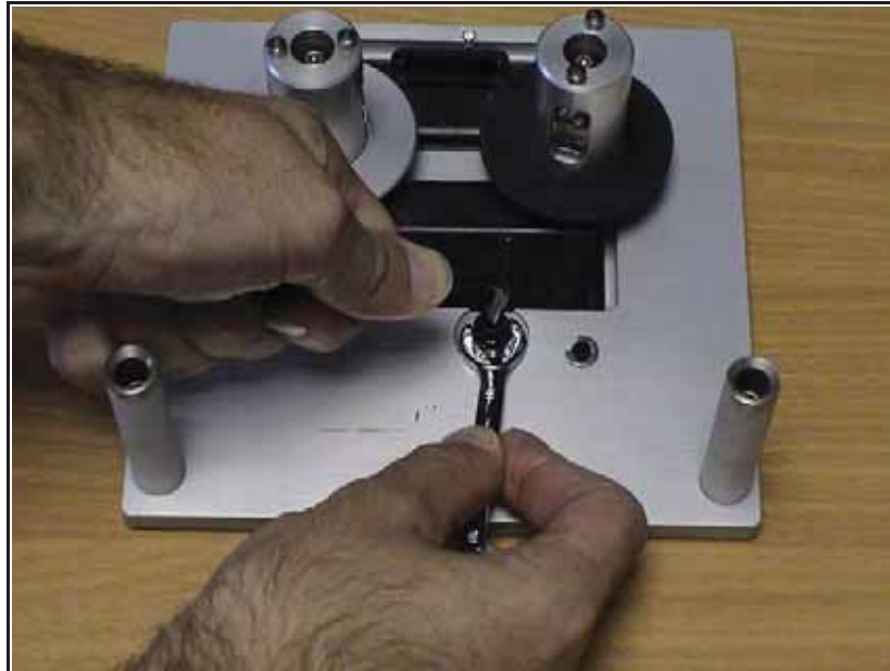
Figure 5-28: Latch Screw Adjustment
