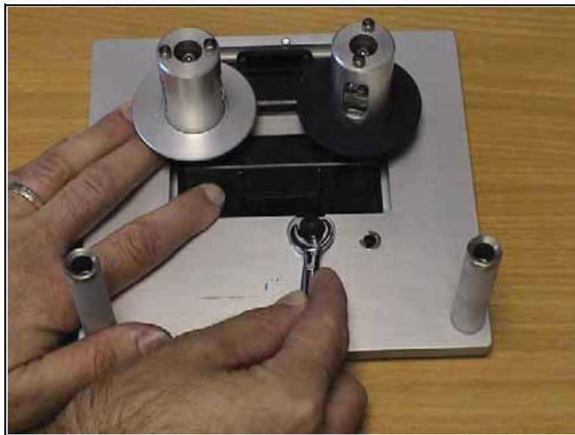
Figure 5-27: Latch Screw Locking Nut Loosening
