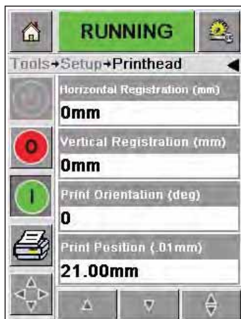
Figure 4-5: Printhead Parameters in Continuous Mode
