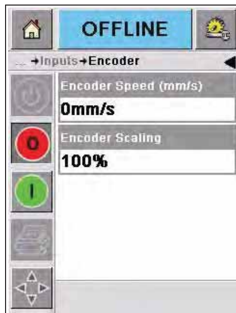
Figure 4-11: Encoder Diagnostics Page
