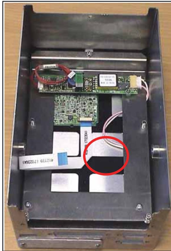
Figure 5-11: LCD Ribbon Cable Detail
