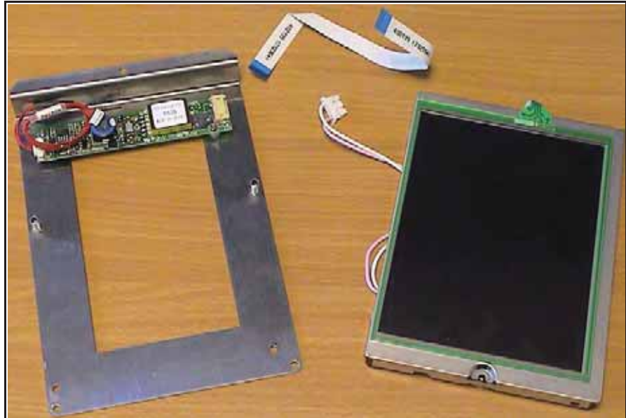
Figure 5-9: Separated LCD Assembly
