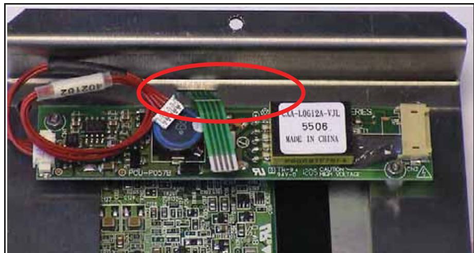
Figure 5-10: Touch Screen Ribbon Cable Routing
